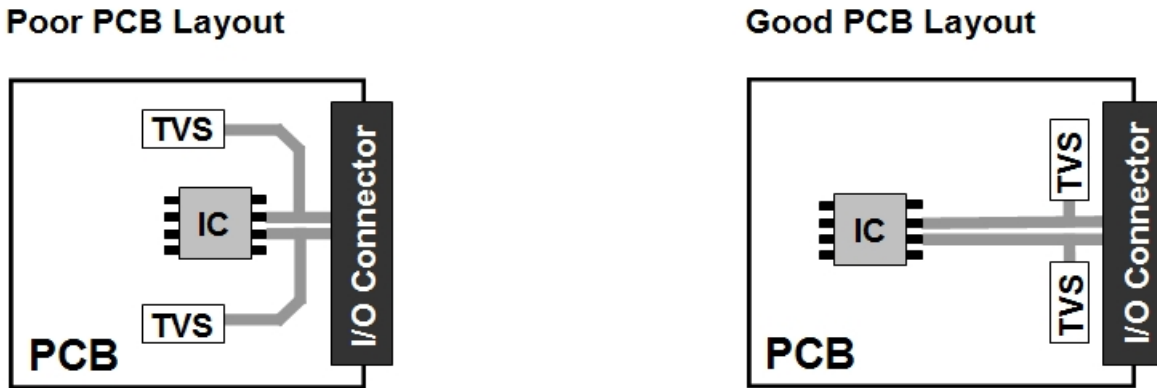
Figure 3. The length of the trace connecting the TVS device to the I/O connector should be minimized and small in comparison with the trace between the connector and IC.
